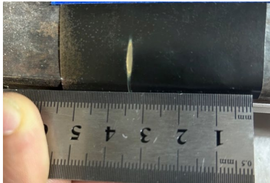
Laser illumination pattern on laser burn paper
