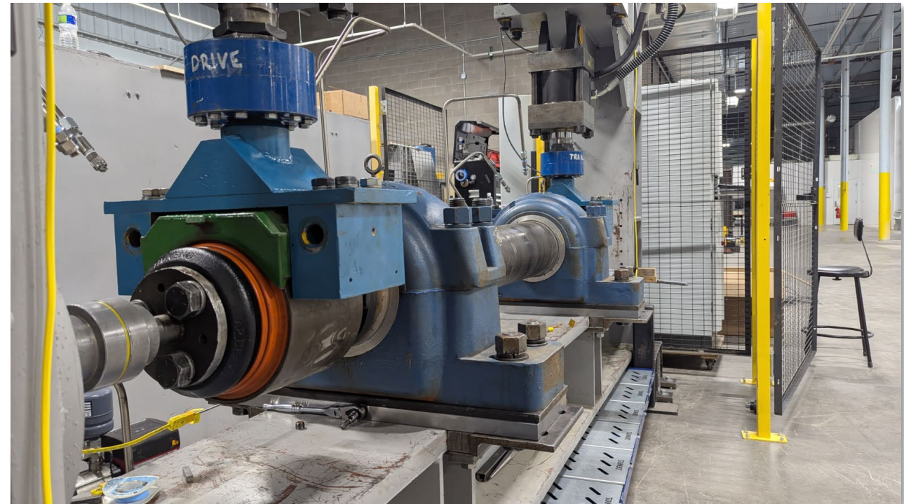
MxV Rail's bearing rig with water spray system
