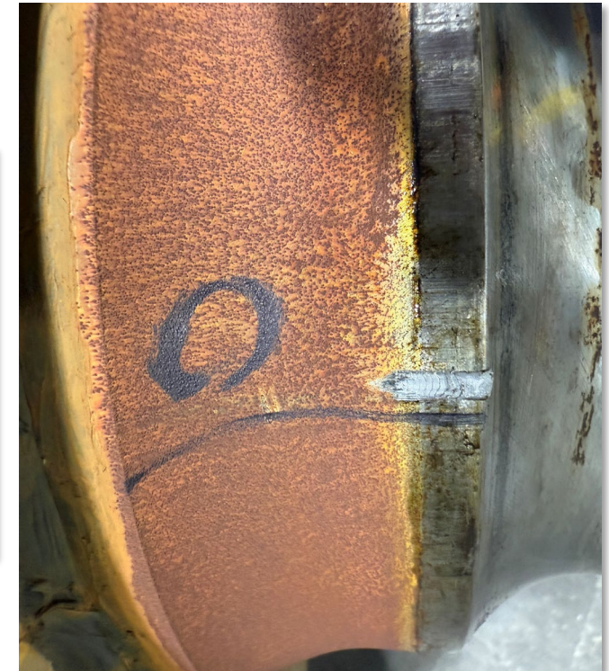
Dust guard gouge left by FBR
