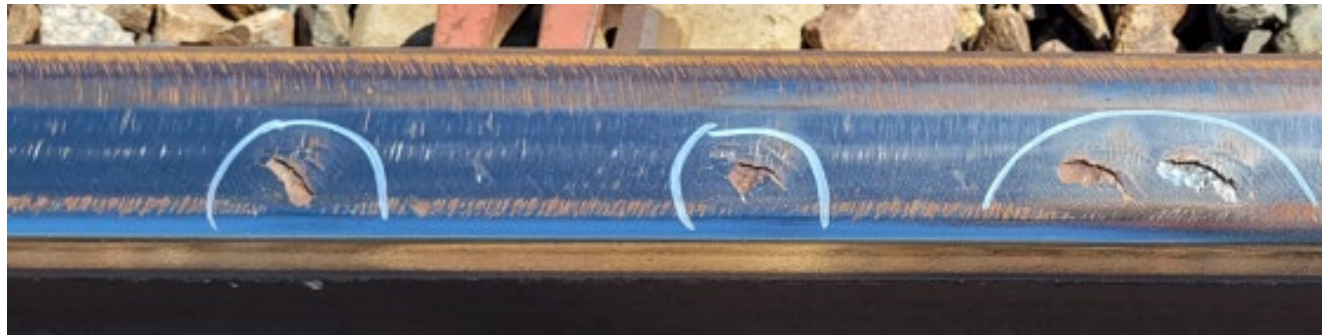
Rail spalls on running surface observed at 1,350 MGT
