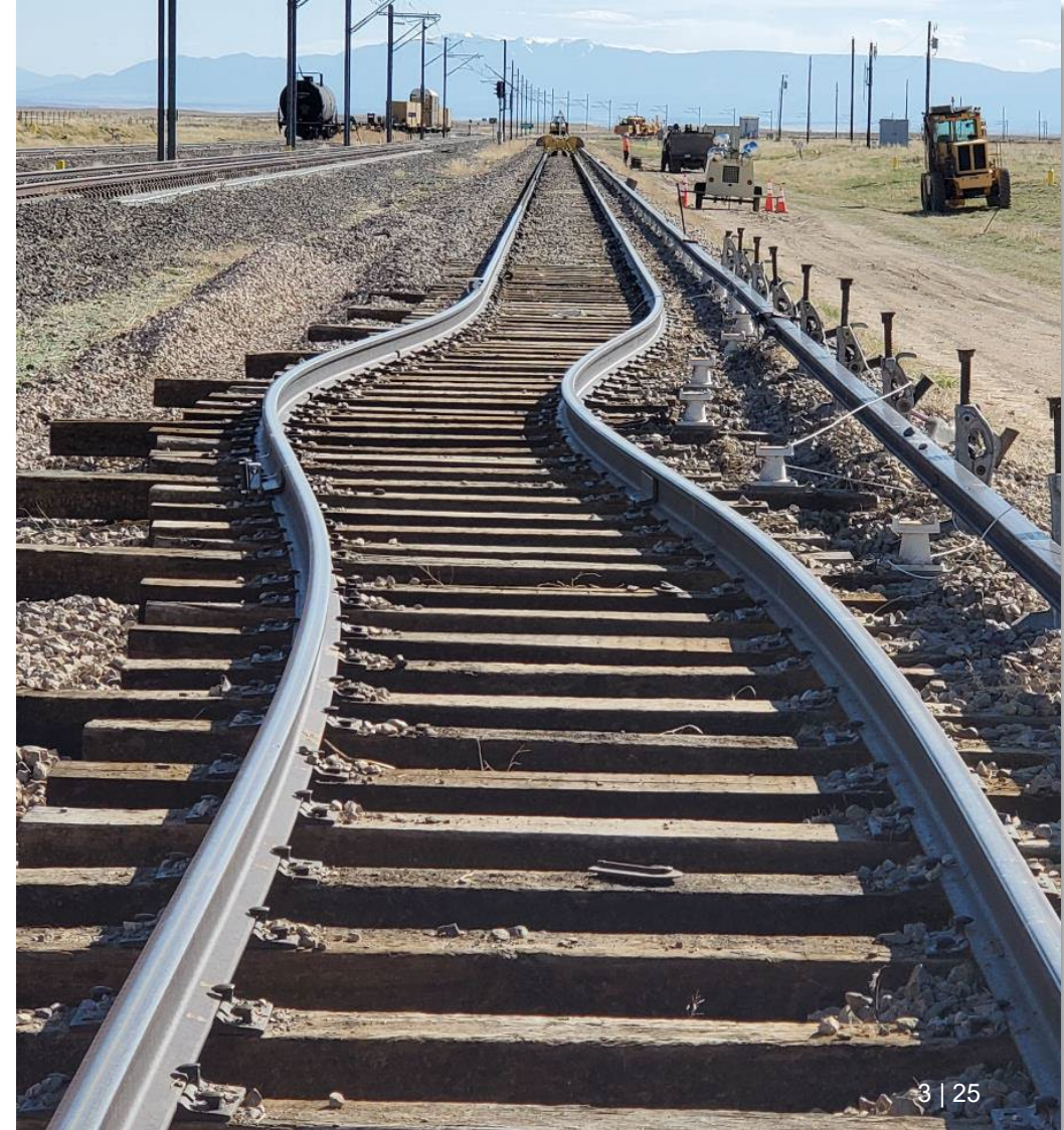
Track Buckle from 2022 MxV Rail/BNSF Test
