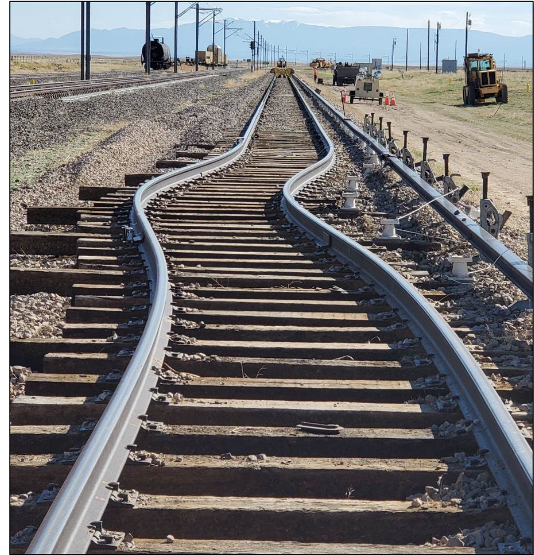
Track Buckle from 2022 MxV Rail/BNSF Test
