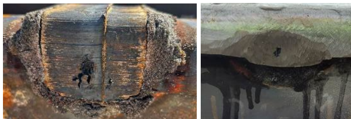
Figure 5. Hot tear defects on the side of the head after a complete shear
