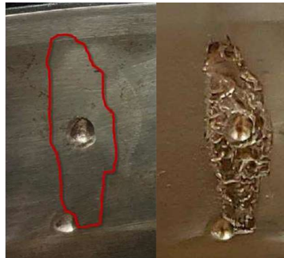
Area around repair spalling during test
