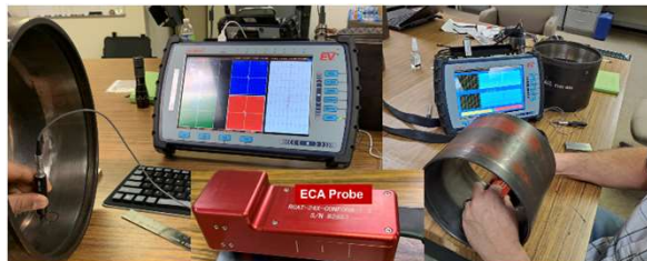
Flexible eddy current array inspection
