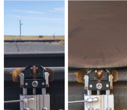
FAST EMAT sensor testing on a sidetrack
