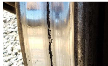
Continuous spalling in wheel
