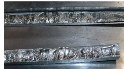
Subsurface fatigue cracks
