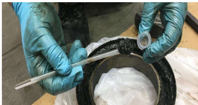
Grease Sampling of Roller Bearing
