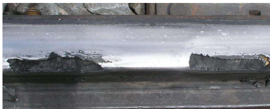
Rail gage corner shelling
