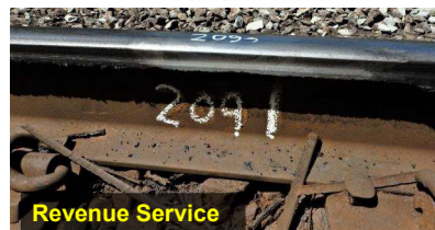
Bottom of gage lip breaking off
