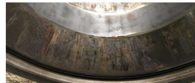
Water Etch on Bearing Raceway 153
