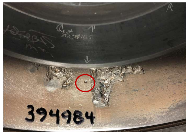
Bearing raceway spall during test
