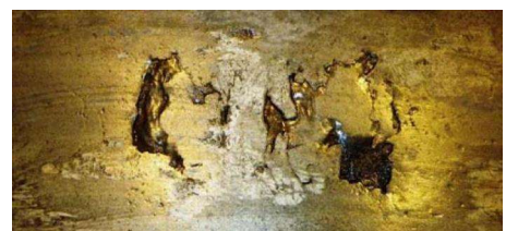
Wheel tread spalling
