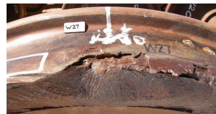
Fatigue defect in wheel tread
