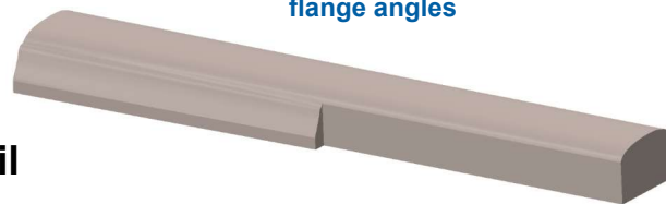
3D CAD model of turnout switch and stock rails
