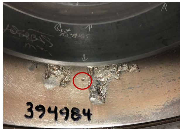
Bearing raceway spall during test
