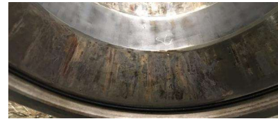
Water Etch on Bearing Raceway
