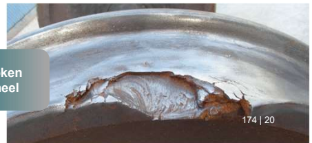
Propagating sub-surface cracks
