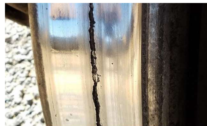
Continuous spalling in wheel
