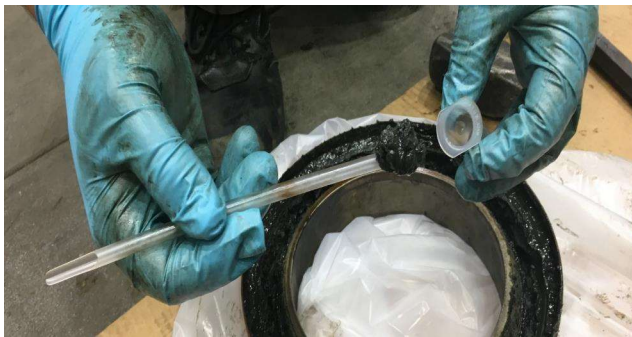
Grease Sampling of Roller Bearing
