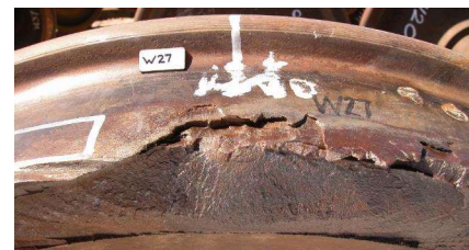
Fatigue defect in wheel tread
