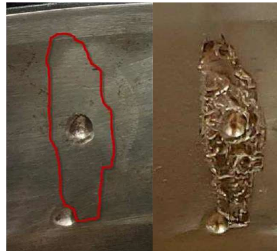
Area around repair spalling during test
