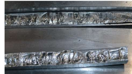
Subsurface fatigue cracks
