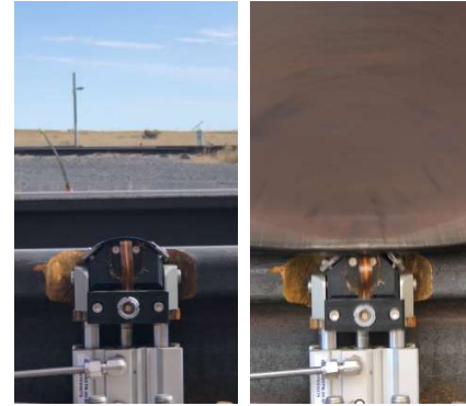
FAST EMAT sensor testing on a sidetrack
