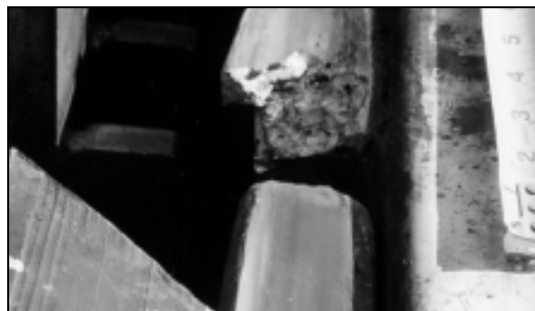
Exhibit 3. Casting Cracking That Caused the Diamond Removal
