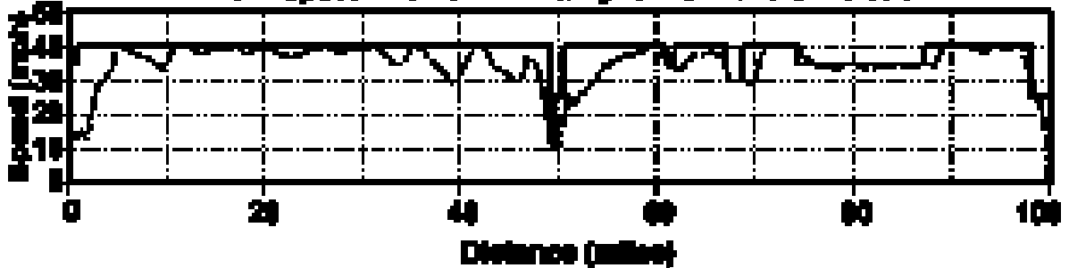
Train Speed Profile — Air & Dynamic Brake Simulation
