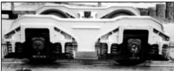
Exhibit 3. The NACO Axle-Motion Truck
