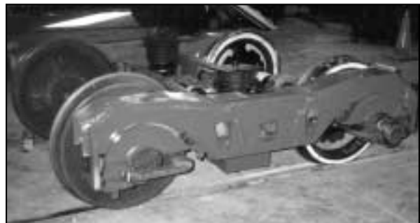
Exhibit 1. GG&W Truck for Bi-Level Auto Rack
