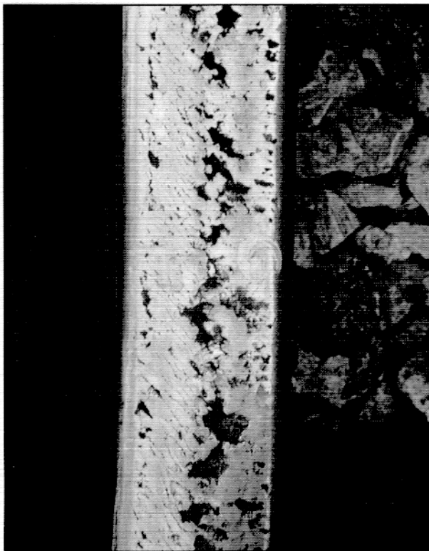
Exhibit 2. Spalling in a "No Grind" Curve. All Grinding Practices with Rodange Rail have Spalled .
