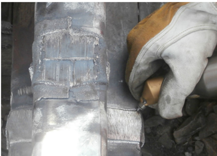
Figure 6. Photograph of the manual UIT process at FAST.
