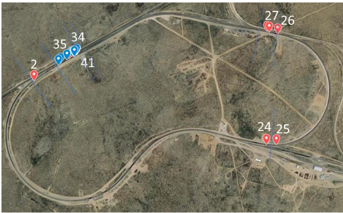
Figure 8. Regulatory geometry defects (red) versus IFC (blue), 87.4 MGT
