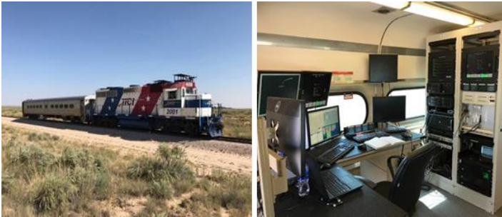
Figure 1. TTCI's rail-bound Track Geometry Measurement Vehicle (TGMV)
