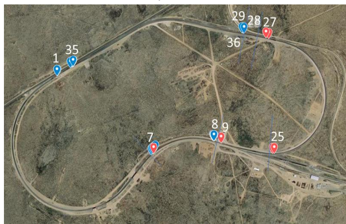
Figure 7. Regulatory geometry defects (red) versus IFC exceptions (blue) at 44.3 MGT
