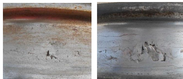
Figure 4. Photographs of RCF tread surface damage on two wheels removed from different cars with disabled brakes
