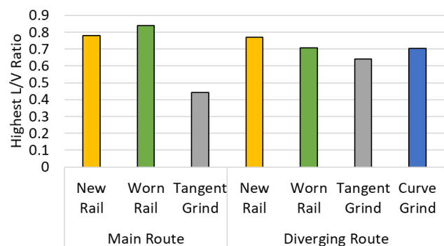
Figure 2. Highest single-wheel L/V values
