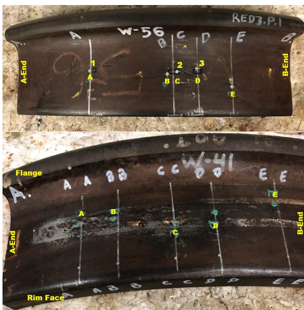
Figure 3. EMAT-detected defects on wheel cut out samples
