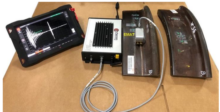
Figure 2. Single channel EMAT test setup
