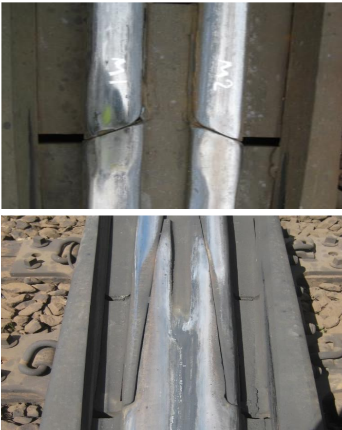
Figure 1. 60-degree convention angle cut heel (top) low impact or tapered heel (bottom)
