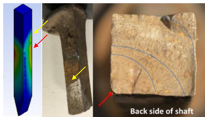
Figure 4. Comparing stress contour from FEA model and actual broken cut spike from revenue service
