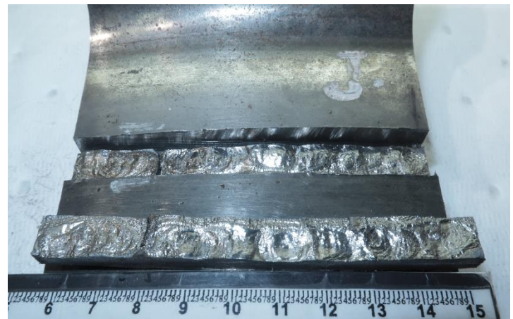
Figure 4. Subsurface fatigue crack found in test wheel
