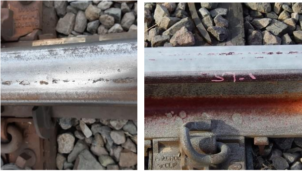
Figure 7. Visual and LPT test result for the low rail in HTL Section 3 at 57 feet location
