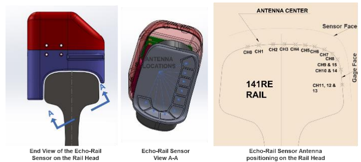
Figure 2. Echo-Rail sensor and antenna placement in the rail head
