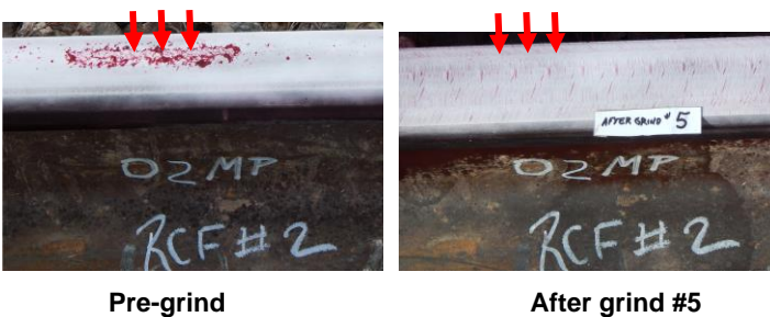
Figure 8. Verification for the high rail at MP2 location. Liquid penetrant results before and after Grind 5
