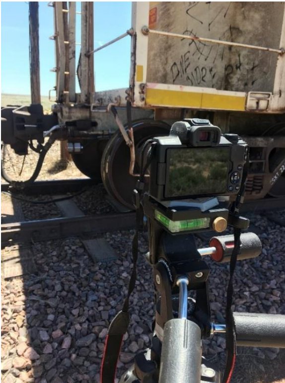
Figure 1. Camera on tripod positioned with respect to top of rail
