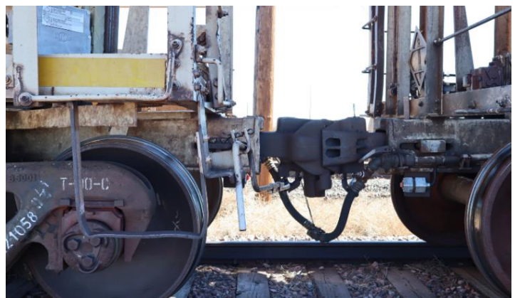
Figure 3. Draft key at camera level, camera 34 inches above top of rail
