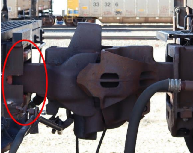
Figure 8. Draft key is obscured when draft system is in the buff position
