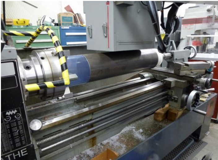
Figure 3. Flash IR hood over a test axle mounted on a lathe to spin at 200 rpm
