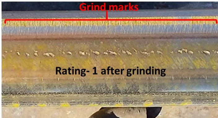
Figure 7. RCF rating of 1 on a type E rail after grinding at 429 MGT and one night of trail operations.
