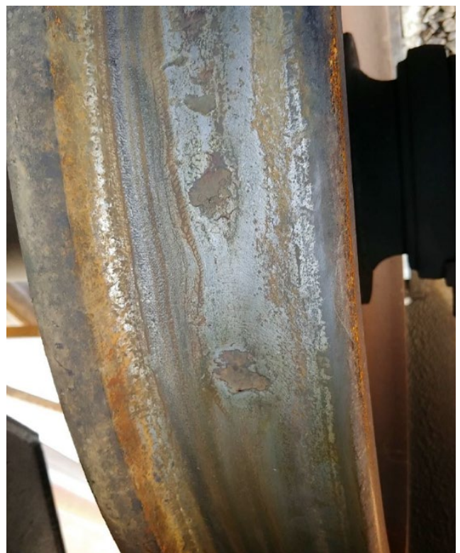
Figure 3. Tread condition of Car W3 Wheel R5 at time of removal
