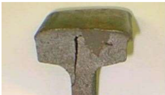
Figure 2. Vertical split head (VSH) defect 2
