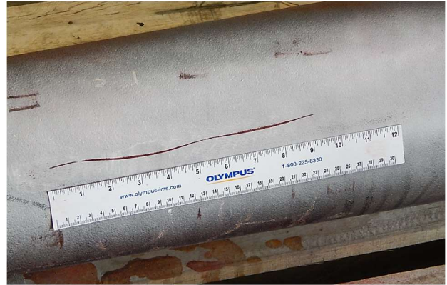
Figure 1. Axle with longitudinal crack with contrast enhanced using magnetic particle testing.
