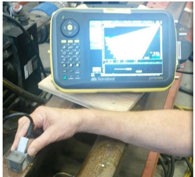
Figure 4. Photograph of the phased array deployed on the railhead
