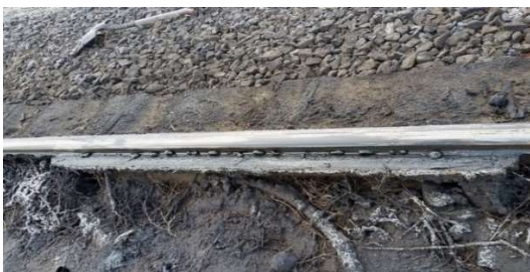
Figure 1. One of two applicator bars of a conventional GF lubrication unit releasing grease with surrounding contamination
