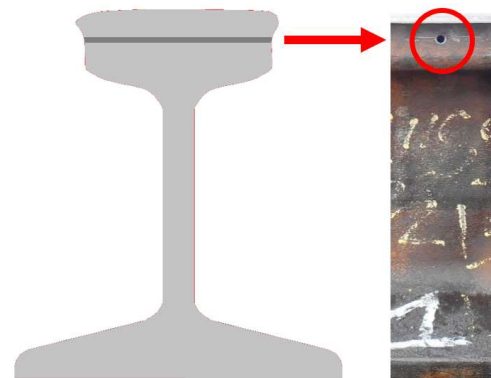
Figure 3. Transverse cross section and side view photo of rail with drilled hole
