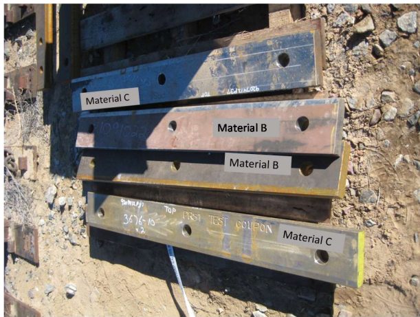
Figure 2. Flange-bearing coupon for FAST evaluation of frog materials
