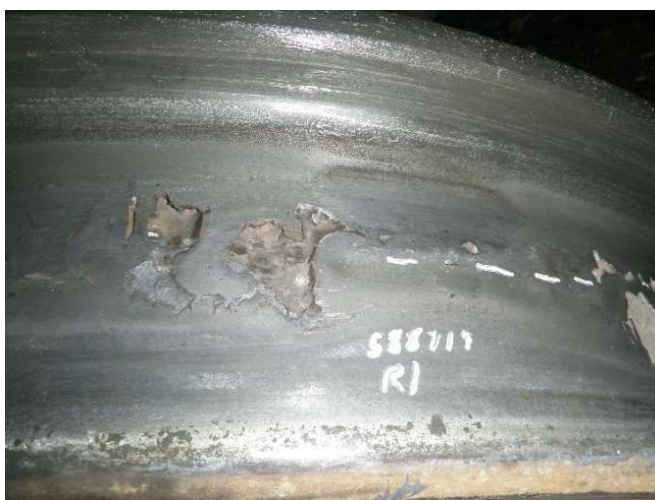
Figure 3. Tread damage on an HPW (317,000 miles).
