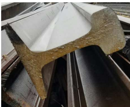
Figure 5. Example of fracture from a base defect
