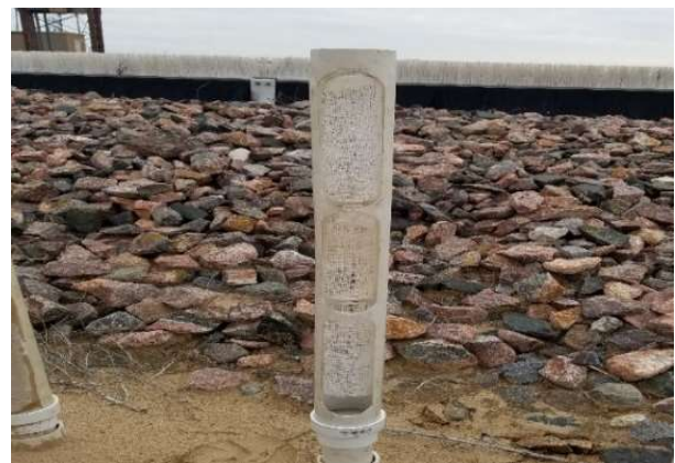
Figure 5. Sand Collection Tube at No. 10 Turnout
