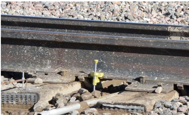
Figure 8. Photograph of Voidmeter
