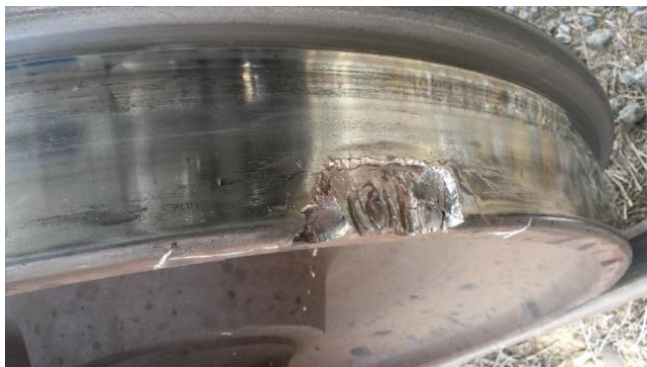
Figure 1. Example Cracked Wheel Damaged near the Rim
