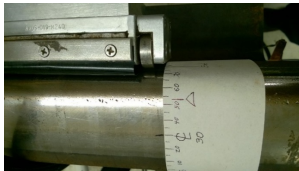
Figure 7. Setup for Scanning Across the Railhead Width. Rail Centerline at 30 mm. Field side is near zero mm
