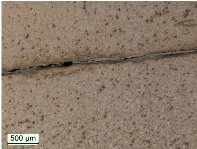
Figure 5. Subsurface Crack with Untempered Martensite in Wheel V8
