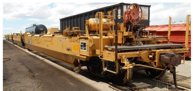
Figure 2. One of the 5-Unit Articulated Well Cars Used in This Test
