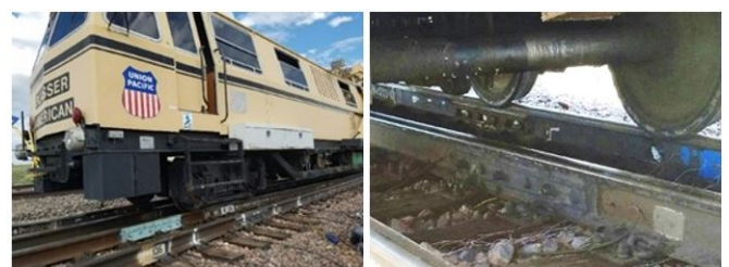
Figure 6. In-field loading experiment showing (left) the welder used to load the IJ, and (right) the wheels loading the IJ
