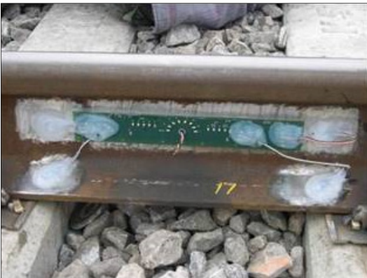
Figure 1. Typical WILD Site Strain Gage Installation
