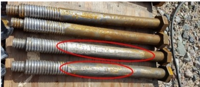
Figure 8. Deformation along the side of the bolts resulting from forced installation by sledge hammer
