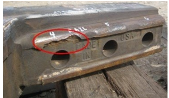
Figure 6. Chipped casting tab that contacts high on the web of the rail at the SW corner
