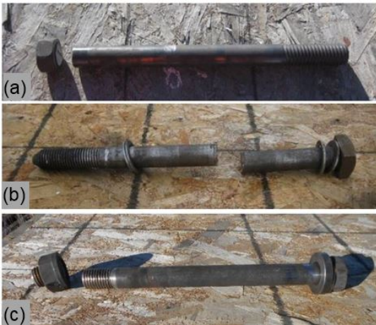
Figure 5. (a) NW Corner, Bolt 3 (Huck 360), 33.23 MGT; (b) SW Corner, Bolt 4 (Copper State), 16.90 MGT; (c) NE Corner, Bolt 4 (LB&N Self-Centering), 12.32 MGT
