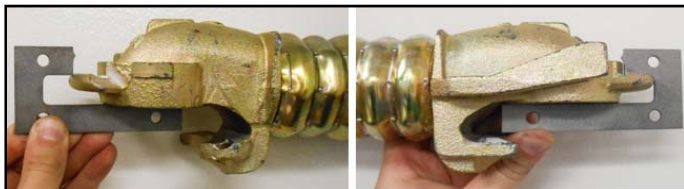
Figure 7. (left) Passed Lip Bead Height Check and (right) Failed Lip Bead Height Check
