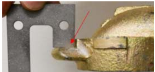
Figure 8. Passed Height Check with Inverted Gauge
