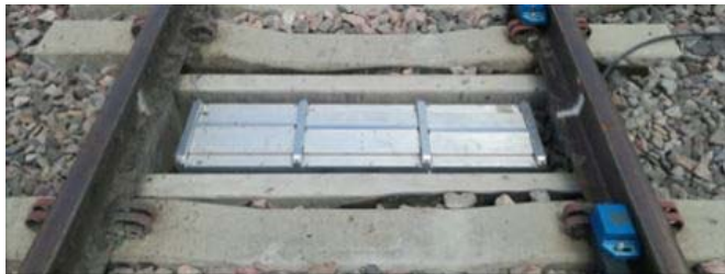
Figure 3. TFDS bottom caisson with between-rail cameras
