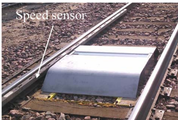
Figure 1. The VUE™ Camera/Lighting Module, and Precision Linear Speed Sensor
