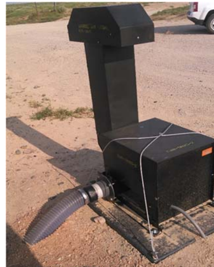
Figure 2. Blower Motor for Air Knife and Cool Air Circulation
