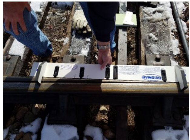
Figure 4 Measuring Gauge Face Wear Angle on an Industrial Turnout
