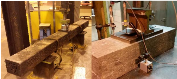
Figure 3. Tie Center Bending Test and Plate Compression Test used to Tune Model Parameters
