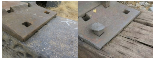
Figure 1. Plate Cutting at the High Rail of (a) An EPC Tie after 1690 MGT and (b) A Control Hardwood Tie after 970 MGT (both installed in a 6-degree curve at FAST)
