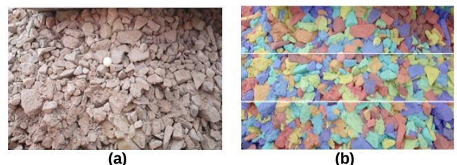
Figure 4. (a) Original trench image (b) Image segmented into colored areas in the three sub-images after processing
