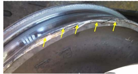
Figure 2. Material Flow at the Rim Face of the Wheel
