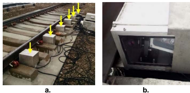
Figure 4. Tread Vision Cameras added to the ACWDS: (a) Six Vision Cameras; (b) Close-up View of the Camera
