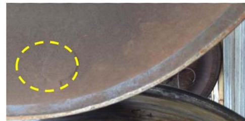
Figure 3. Example of Casting Riser on the Wheel
