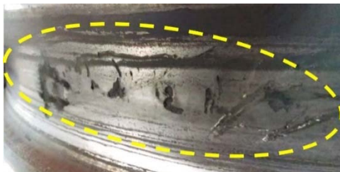
c. Spalled Wheels
