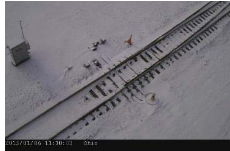
Figure 3. Snow and Ice in Switch Point
