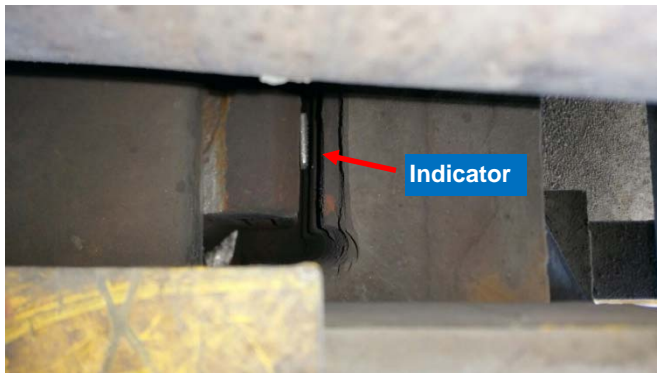
Figure 5. Indicator Magnets after Two Nights of Operation
