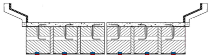
Figure 1. HCB Cross Section Showing Strain Gage Locations
